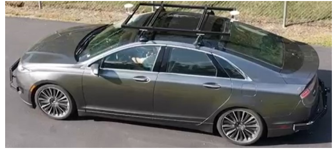
Fig. 3. The AV testing platform, which is a full-size sedan equipped with a drive-by-wire system, a Polynav 2000P GNSS-inertial system, a Calmcar front view camera with lane detection capabilities, and a Dspace Autera computing unit.
