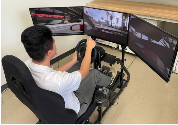
Fig. 5. The driver-in-the-loop simulator with CARLA used by Driver 1 & Driver 2.
