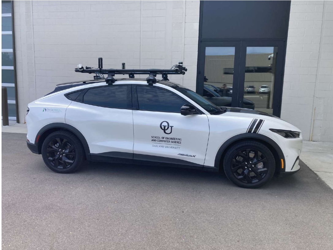
Figure 3.1: Ford Mustang Mach-E for on-road LiDAR data collection.
